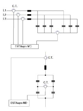
The double star circuit generates a sum current the size and phase of which result from the three unbalance currents. Using the reference current, the ESTAsym MD can analyze the sum current into the three unbalanced currents. Each change of the sum current can take place only in the same phase of the capacitor current. Thus the ESTAsym MD can reveal the partial path in which the defective capacitor unit is located. This means that only 1/6 of the capacitors need to be checked.
